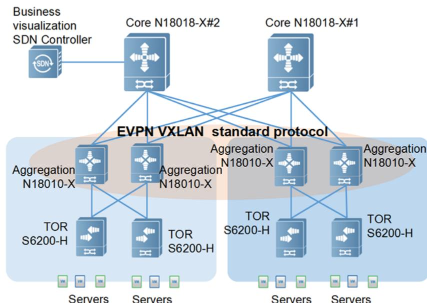
Figure 6: Typical Application of the RG-S6220H Switch Series
