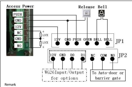
If let relay drive electric - lock, please connect a reverse diode with the lock's "+" and "-" poles.
