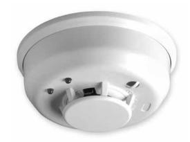
Honeywell's 5808W3 is a 3V lithium powered, photoelectronic smoke/heat detector with a built-in wireless transmitter. It is intended for use with any 5800 Series Wireless Receiver/Transceiver for residential installations (for commercial installations, the 5881ENHC or the 5883H receiver is required).
