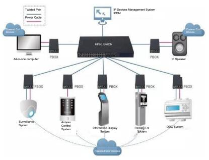
Figure 5: RG-S2910-H Powering the End Devices
