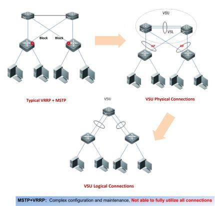
VSU: Simple configuration, does not require VRRP and MSTP, all connections are utilized
