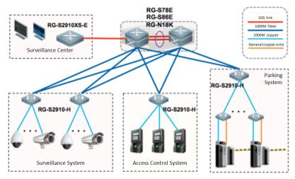
Figure 4: RG-S2910-H Deployment for Smart Building
