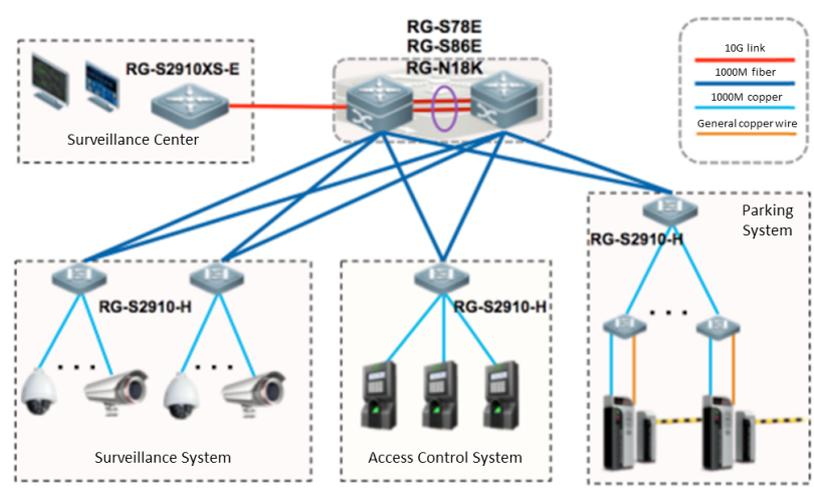
Figure 4: RG-S2910-H Deployment for Smart Building
