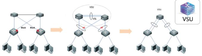
**MSTP+VRRP** : Complex configuration and maintenance, **Not able to fully utilize all connections**
