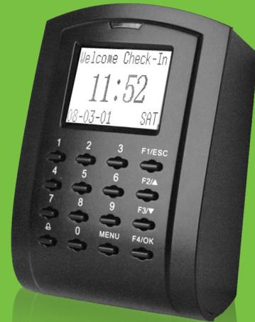
SC103 is an access control device produced by ZKTeco, which is made with elegant design and professional surface treatment. The device has lock control, alarm, exit, button and door sensor. The wiegand-in interface is used to connect external reader to construct master and slave system. Also, the device can be used to connect with a control panel as a
