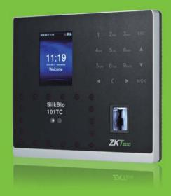
SilkBio-101TC is Time & Attendance and Access Control Terminal to be associated with SilkID fingerprint reader, face recognition and RFID card functions. With the new SilkID fingerprint reader, the operation remains stable under strong light source and high preciseness of verification of wet and rough fingers. With latest facial algorithm and the innovation features, Silkbio-100TC is bringing you the whole new experience.
