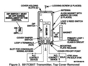
**NOTE:** For UL commercial and household fire installations, only one initiating device may be connected to this transmitter. For UL commercial burglary installations, multiple initiating devices may be used as long as the devices all service the same function such as door/window contacts, motion or glassbreak detectors. All initiating devices must be located within the same room. No more than one wire per terminal may be connected. Use only 14-22AWG wire.
