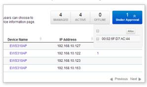
This screen in the interface displays the status of all Neutron Series Access Points that your Controller is currently managing as well as all the Neutron Series Access Points in the network that have been discovered. IT managers can add Neutron Series Access Points to the Neutron Series Controller Access Point list.
